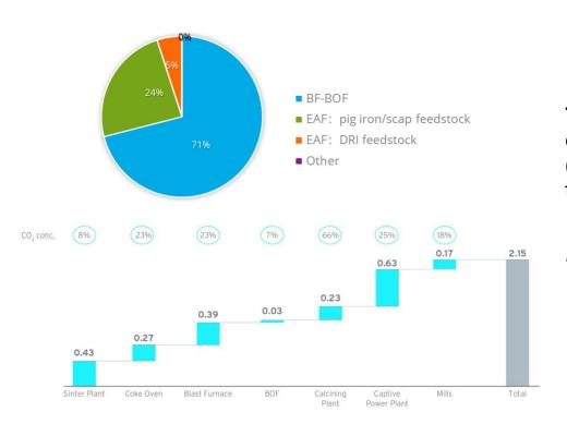
**70**% of the world steel production is based on Blast Furnace – Basic Oxygen Furnace (BF-BOF) route, that has a strong impact on the CO<sub>2</sub> production.
