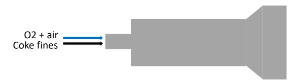
Flame evaluation: heterogenous kinetic, semiempirical data The O2 flow rate was recalculated to achieve **stoichiometric oxygen** in the combustion chamber.
